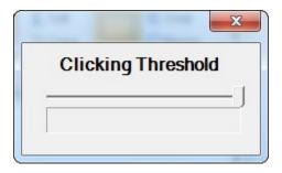
The blue bar represents the amount of eyebrow motion detected. This motion is used by our system to generate mouse clicks. The knob pointing down on the blue motion bar is the slider.
